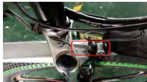
Fix the front Fender The front fender and front light share the same hole on the fork
