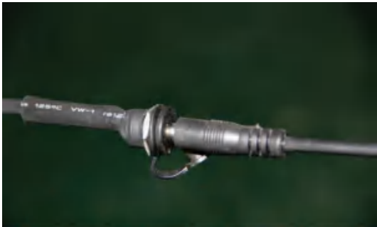
Connect the Battery Cabel and the charger Cabel
