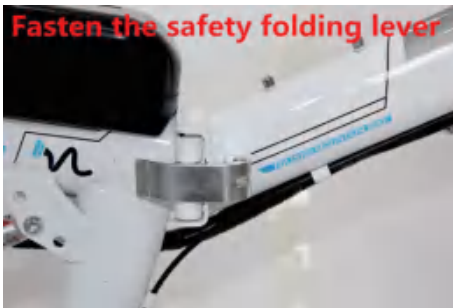
Turn the folding lever on the handle post
