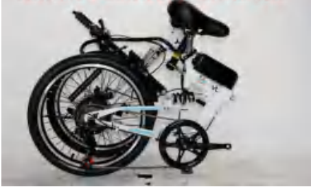
Fasten the safety folding lever
