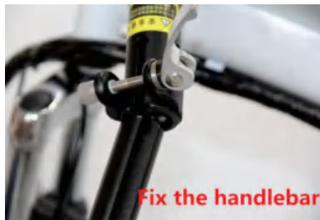
Fasten the folding lever on the handle post
