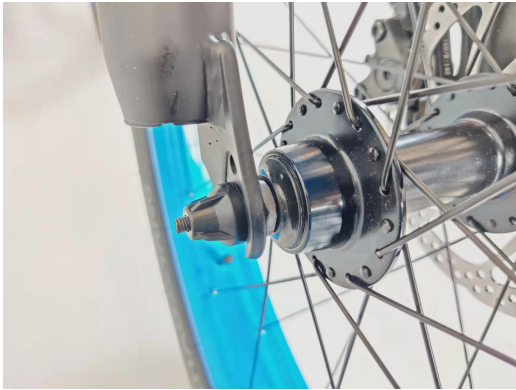
19. Tighten the nut on the other side
