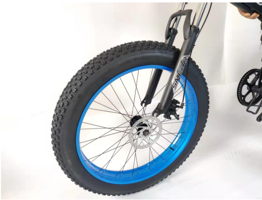
13. Put the front wheel between the legs of the fork
