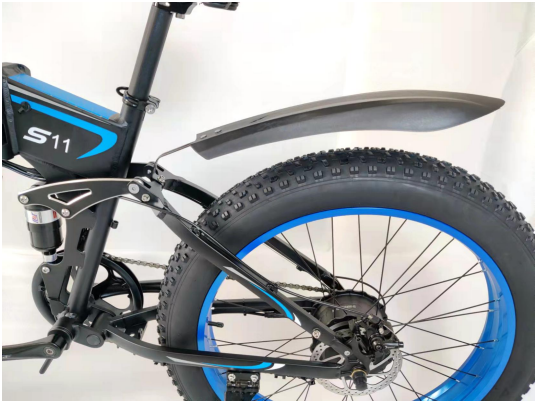
31. Rear fender installation completed
