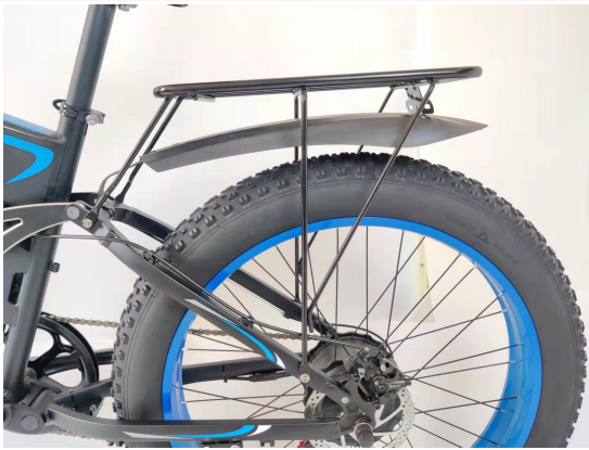
37. Rear rack installation completed
