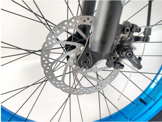
15. The fork dropouts hold the tips of the front hub
