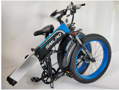
49. The battery can be charged inside or outside the frame
