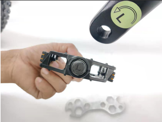
39. The pedal with letter L should be fixed on the left side
