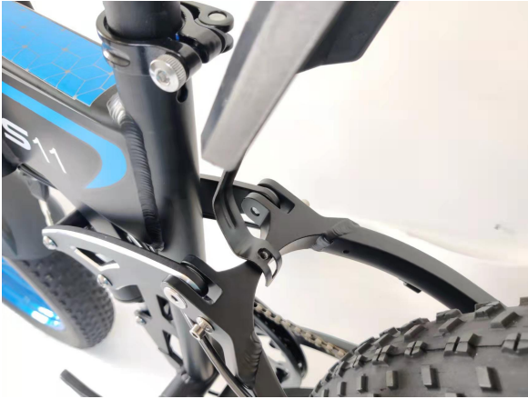
29. The correct placement method of rear fender
