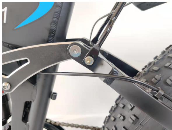
34. Tighten the 2 bolts on both sides
