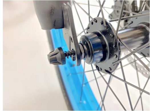
18. The nut and spring on the other side
