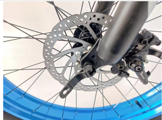
20. Turn the lever of the QR clockwise to tighten it
