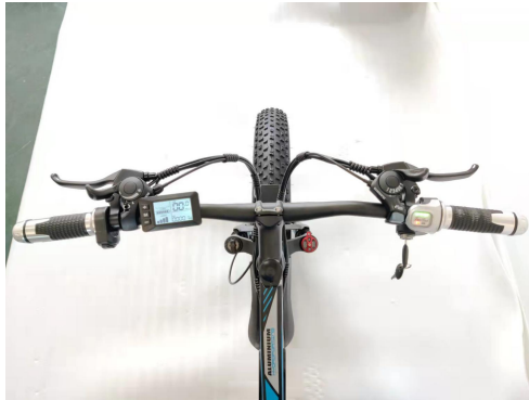
51. Turn the key on the handlebar first and then press button M for 3 seconds on the display to turn on power.
