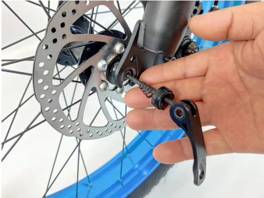
17. Insert the QR skewer into the axle hole of the front hub
