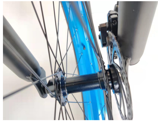
14. Insert the disc rotor into the gap of front brake caliper
