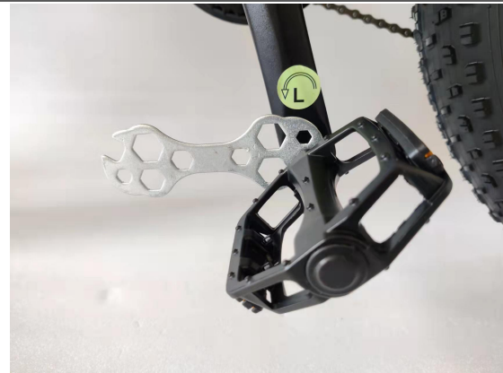
40. Turn spanner counter-clockwise to fix the pedal L
