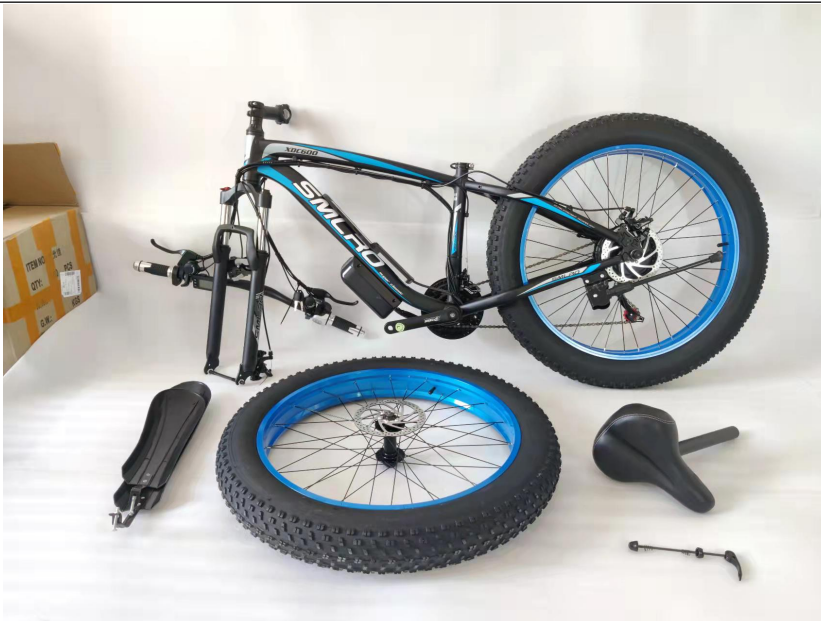
03. Only need to install front wheel, handlebar, saddle, fenders, battery and rear rack
