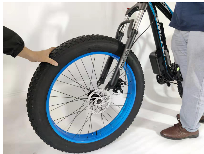
16. Put the front wheel between the two lower legs of the fork
