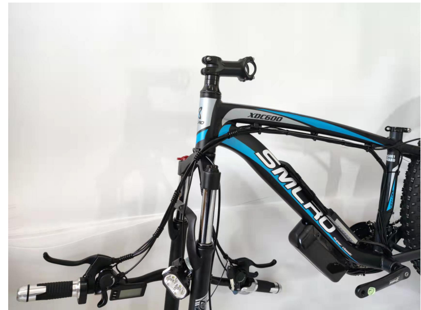
04. The arch of the fork should be facing forward
