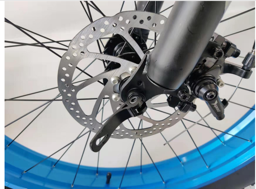
21. Turn the lever of the QR clockwise to tighten it
