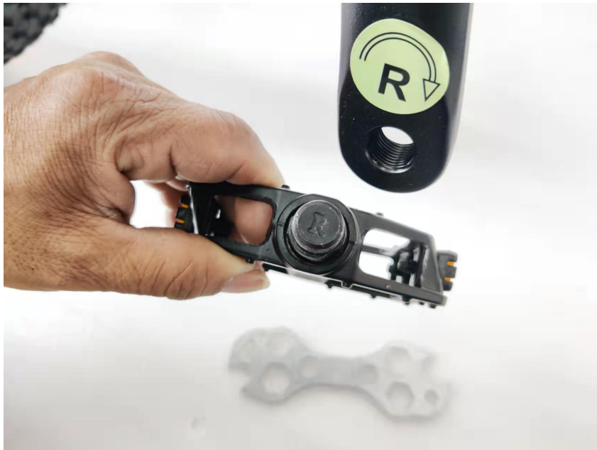
40. Turn the spanner clockwise to fix the pedal R on the right side
