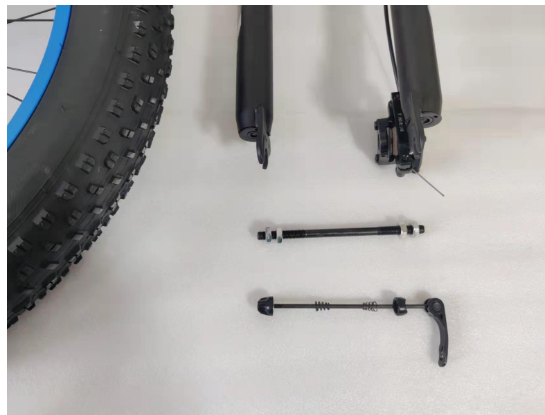
14. Remove the fork spacer. (it protects the fork from crushing and deformation during shipping, it is not a part of the bike )
