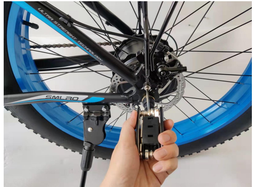
38. Tighten the 2 lower bolts on both sides
