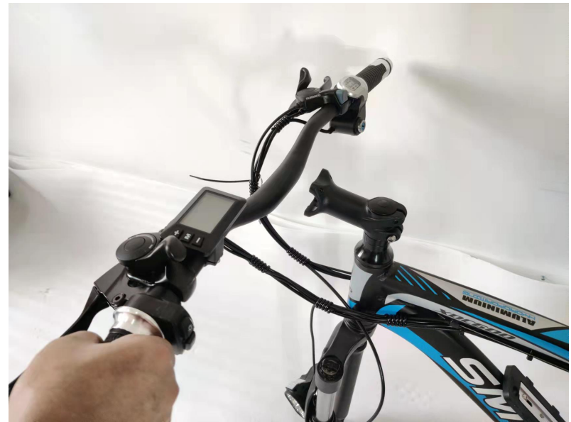
08. The correct orientation of the handlebar
