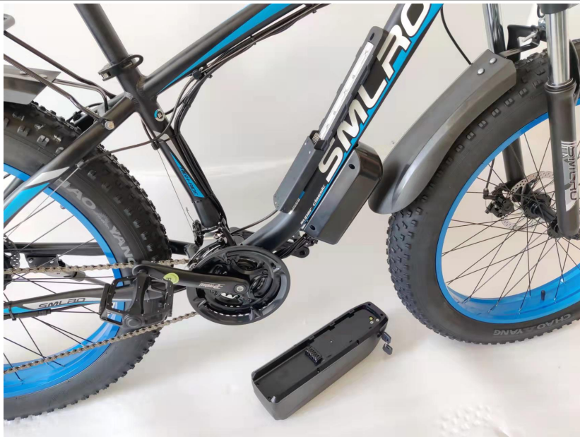
41. Put the battery on the battery base
