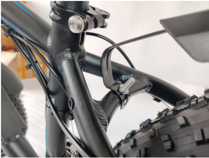
32. Fix rear fender to the frame with bolt and nut
