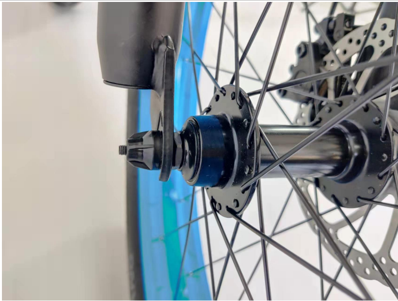
20. Tighten the nut on the other side
