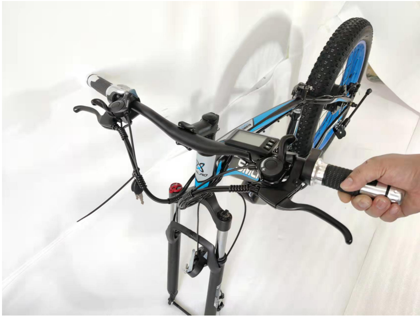
09. Fit the stem and handlebar together
