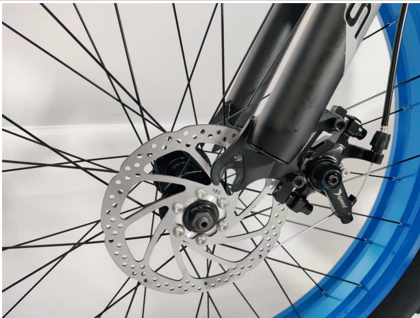
17. Insert the disc rotor into the gap of front brake caliper
