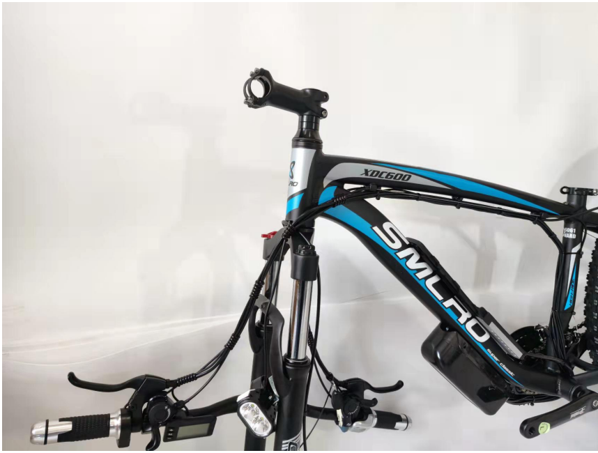
05. Turn the stem forward ( do not turn the whole fork )
