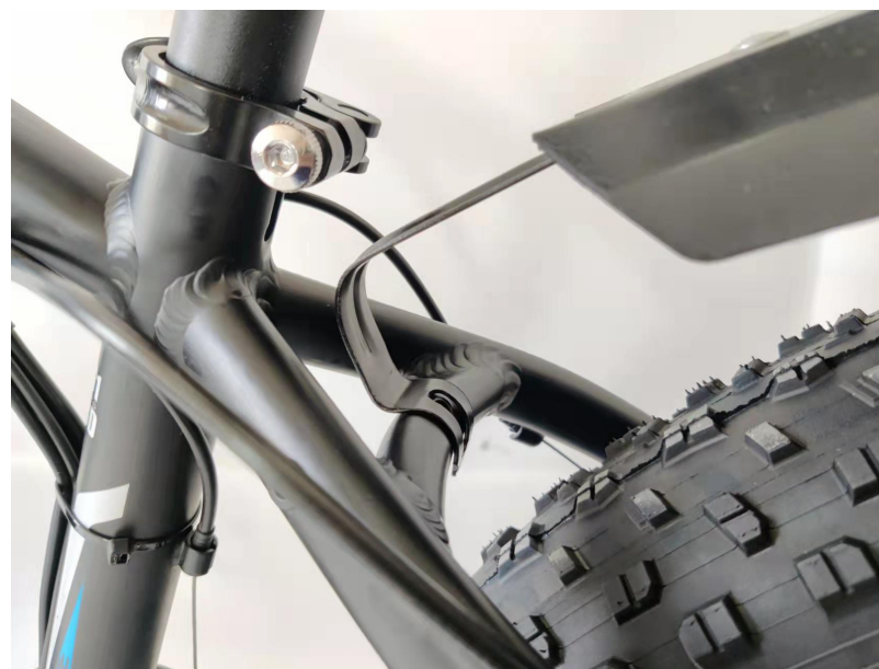
31. The correct placement method of rear fender
