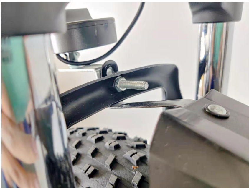
28. details of the bolt that join headlight and fender together
