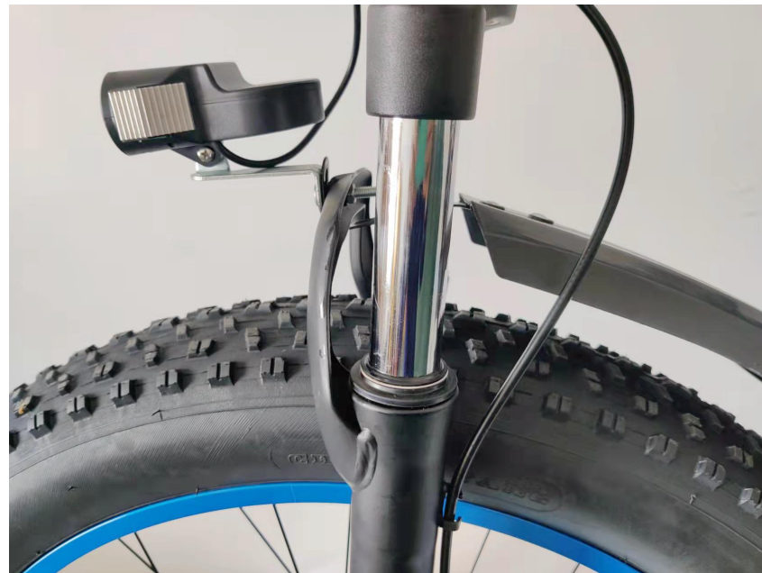
29. The headlight and fender are fixed to the fork arch
