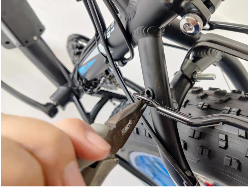
36. Adjust the angles of the rack sticks with sharp-nose pliers
