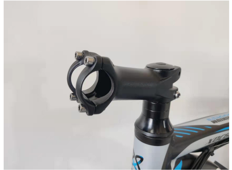
06. The correct direction the stem should be facing
