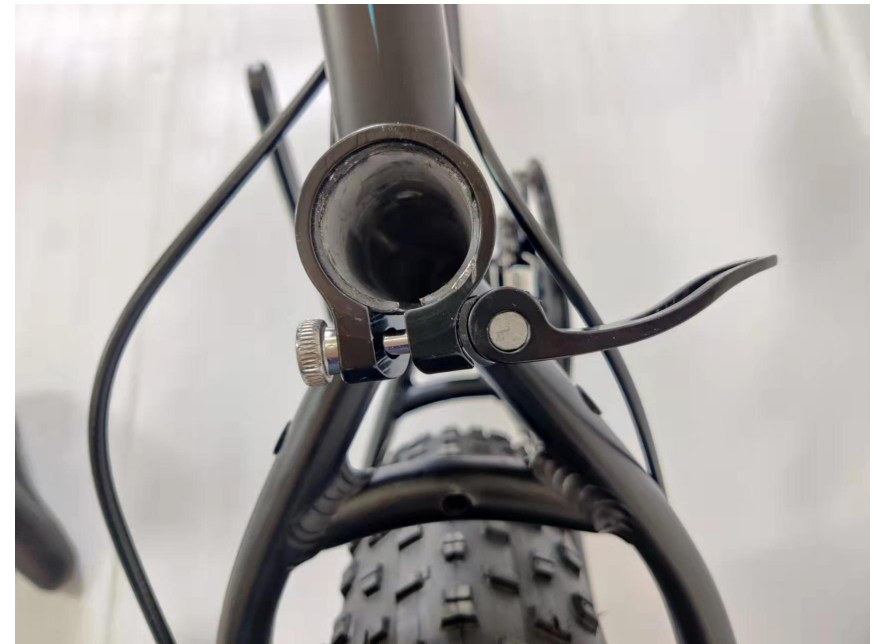
23. Open the lever and turn the nut to loose the seat post clamp
