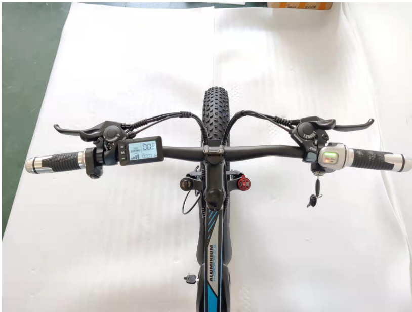
45. Turn the key on the handlebar first and then press button M for 3 seconds on the display to turn on power.
