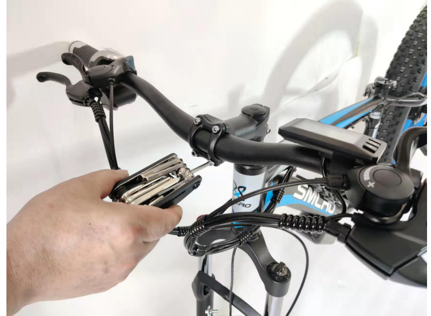
10. Tighten the 4 bolts to fix handlebar
