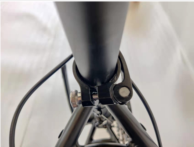
24. Insert the seat post into the seat tube
