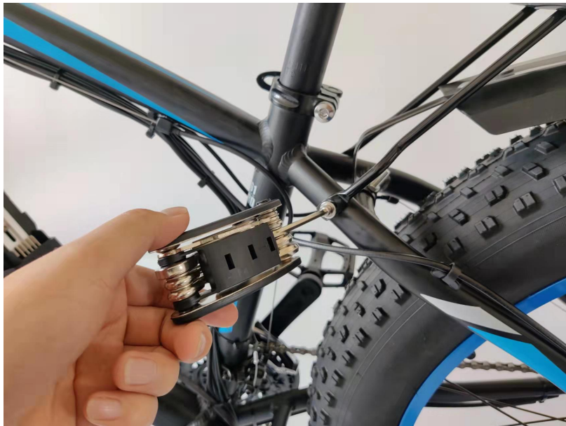
37. Tighten the 2 upper bolts on both sides
