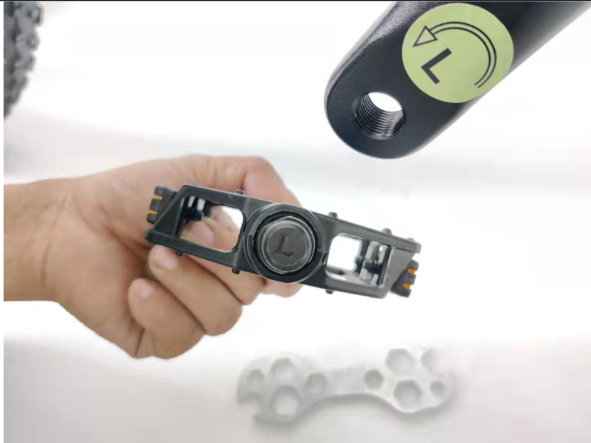
39. Turn spanner counter-clockwise to fix the pedal L on the left side
