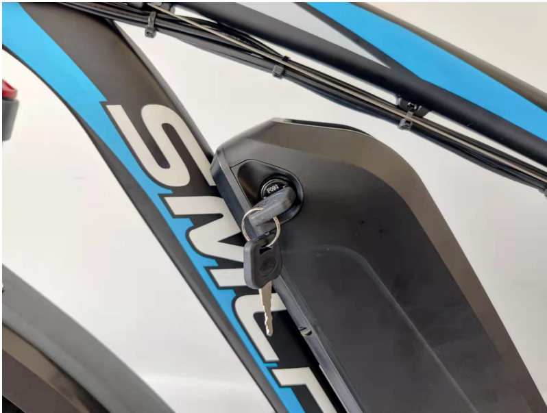
43. Turn the key to lock the battery
