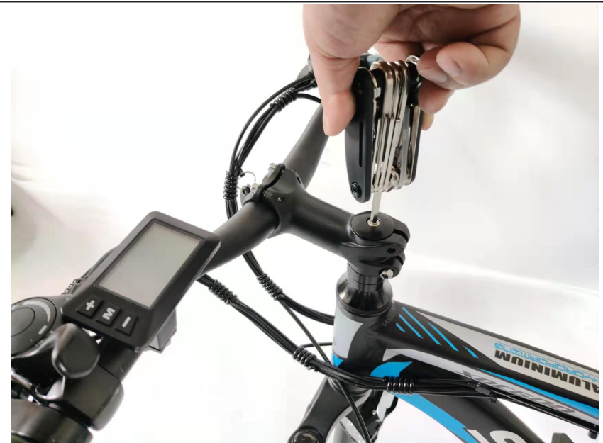
12. Tighten the top bolt
