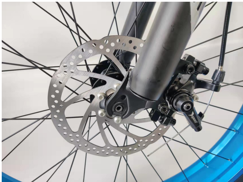
18. The fork dropouts hold the tips of the front hub
