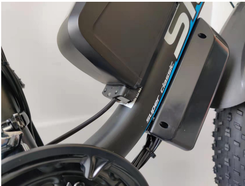
42. Push the battery downward to install it tightly
