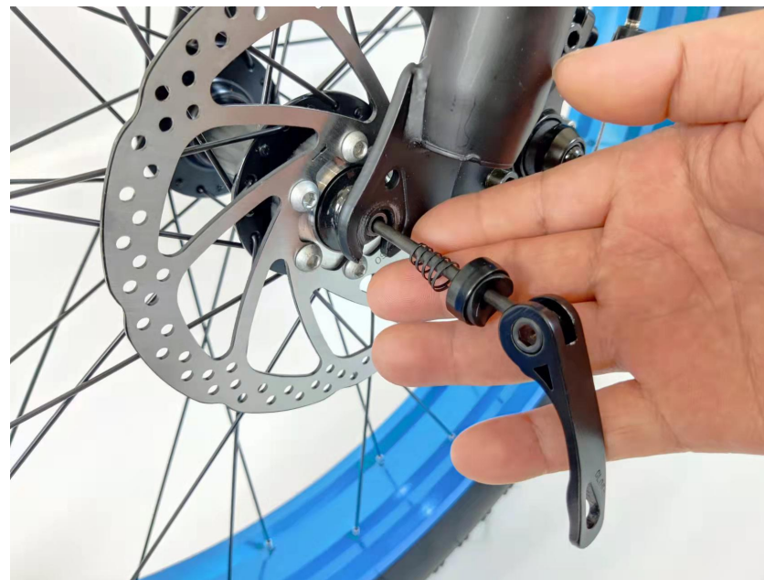
19. Insert the QR skewer into the axle hole of the front hub
