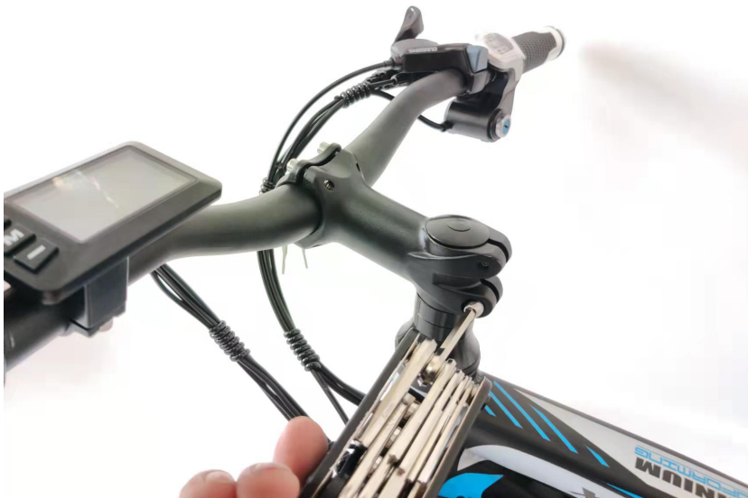
11. Turn the 2 bolts on both sides to tighten the stem
