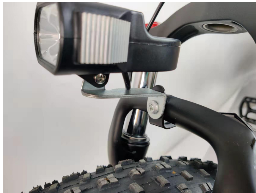
27. Use the long bolt to join the headlight, fork arch and fender
